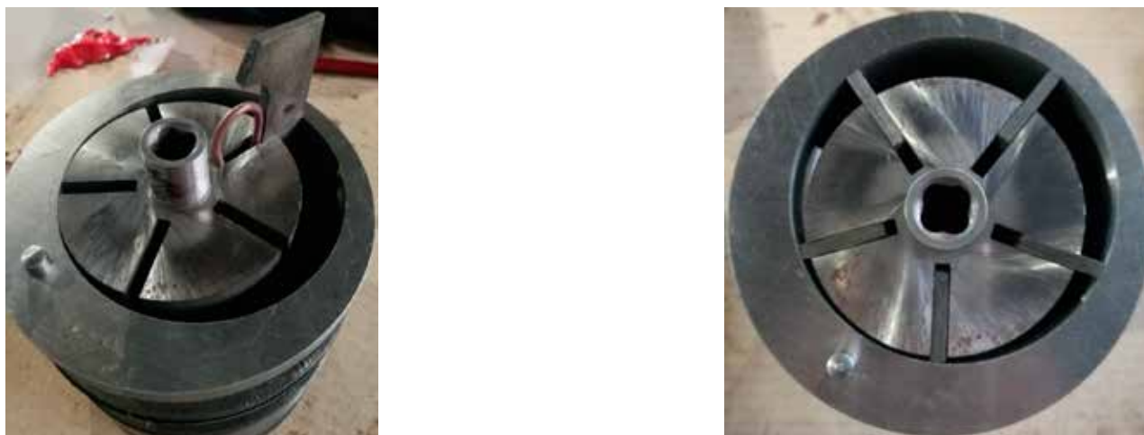
Figure 5: Rotor Vanes and O-Rings
