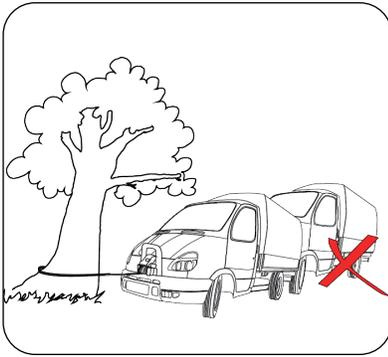
1. Do not exceed winch or winch rope rated capacity.
