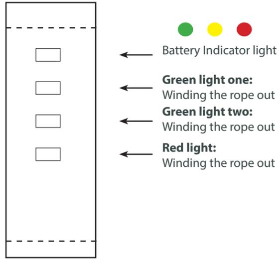
1. Press the power switch (“ON”) of pulling tool, the display light is on. Press the direction switch “▲”, “the green light one” light up, pulling tool is releasing the cable. Press the direction switch “▼” “the green light one” go out and “The green light two” light up. Pulling tool is in the winding mode.
