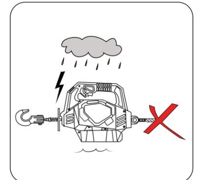
6. Do not submerge winch in water. Always store the remote control in protected, clean, dry area.
