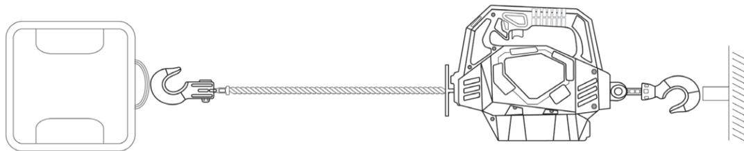
2. Install the battery. Make sure the position of power switch is at "OFF /O". Put the battery into this product, ensure the latch is fully engaged.
