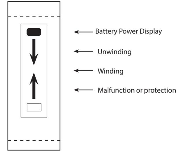
1. Display of battery power: five greeds are green. When the battery displays only one grid, please charge it soon.
