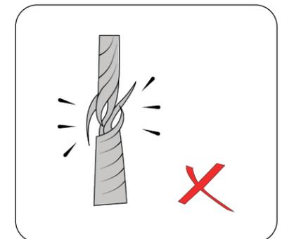
3. Always inspect winch rope, hook, and slings before operating winch. Frayed, kinked or damaged winch rope must be replaced immediately.
