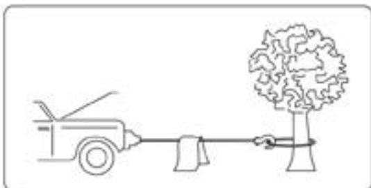
Step 12: Operate winch and pull. Check winch regularly to ensure that wire rope is wrapping evenly onto drum. If necessary unroll cable again and roll evenly. Repeat until vehicle is recovered. Avoid pulling in sharp angles.
