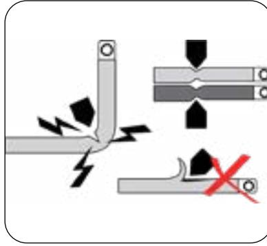
**2.** Do not route electrical cables across sharp edges, near parts that get hot and/ or through or near-moving parts.
