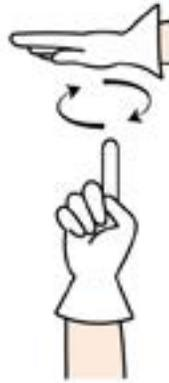
Pull slowly: With forearm in vertical position and forefinger pointing up, move hand in small horizontal circles while other hand stays horizontal motionless.
