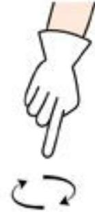
Unwind: With arm extended downward and forefinger pointing down, move hand in small horizontal circles.
