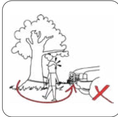
**5.** During winching operation always be aware of stability of vehicle and load during winching, keep others away. Alert all bystanders of an unstable condition.
