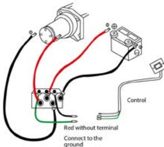
Solenoid box for PWLD3000Ai12/24V - PWLD4000A12V - PWLD600012V (refer to Fig. 9)
