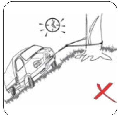
**9.** Do not leave loads unattended, wire rope could come loose from the drum, as the wire rope attachment to the drum is not designed to hold a load.
