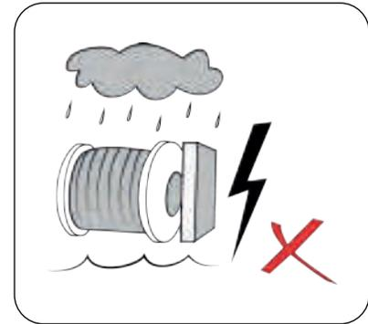
**6.** Do not submerge winch in water. Always store the remote control in a protected, clean, dry area.
