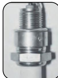
Remove the carbon attached to the electrode, polish the electrode with emery paper, and adjust the electrode gap.
