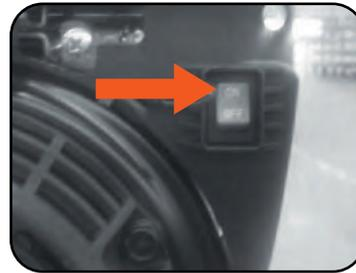
Push the engine switch to the ON (I) position.
