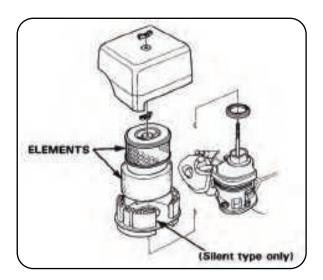
Never run the engine without the air cleaner. Rapid engine wear will result from contaminants, such as dust and dirt, being drawn through the carburetor and into the engine.
