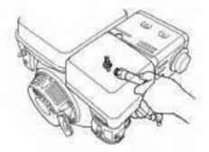
5. After the spark plug is seated, tighten with a spark plug wrench to com- press the washer.
