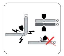
2. Do not route electrical cables across sharp edges, near parts that get hot and/ or through or near moving parts.
