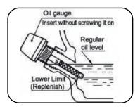
Be sure to check the amount of oil before each operation and fill the reservoir to the proper level. Change the oil if it is dirty.
