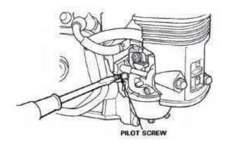
3. After the pilot screw is correctly adjusted, turn the throttle stop screw to obtain the standard idle speed. Standard idle speed:  $1400 \pm 150$  rpm.
