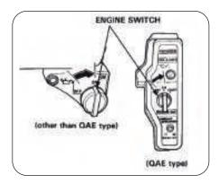
4. Start the engine. With recoil starter. Turn the engine switch to the ON position.
