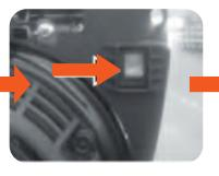
Push the engine switch to the OFF (0) position or tum the key switch to the OFF (0) position.
