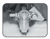
Remove the strainer cup of fuel cock, remove the deposit in the cup and clean the net.
