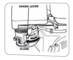
2. Move the choke lever to the **CLOSE** position NOTE: The choke may not be need ed if the engine is warm or the air temperature is high.
