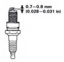
4. Check that the spark plug washer is in good condition, and thread the spark plug in by hand to prevent cross-threading
