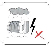
6. Do not submerge winch in water. Always store the remote control in aprotected, clean, dry area.
