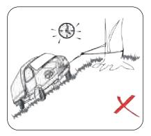
9. Do not leave loads unattended, wire rope could come loose from the drum, as the wire rope attachment to the drum is not designed to hold a load.
