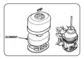
Check the air cleaner element to be sure it is clean and in good condition. Clean or replace the element if necessary (p. 23).
