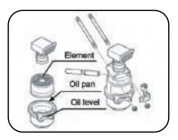
When the oil level is low, add oil to raise it to the correct level. When the element is very dirty, wash the oil pan and the element with kerosene, soak the element in engine oil, and shake or wring it until dripping stops.
