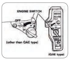
2. Turn the engine switch to the OFF position.
