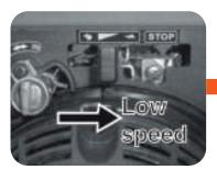
Move the speed control to the slow position and keep the engine running for 1 or 2 minutes.
