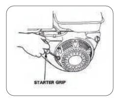
Pull the starter grip lightly until resistance is felt, then pull briskly.
