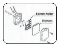
When the element is dirty or the oil has run out, dry the element, soak it in kerosene, vigorously wring out element with one hand.
