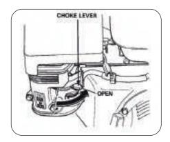
1. As the engine warms up, gradual ly move the choke lever to the OPEN position.
