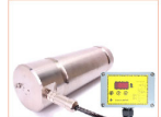
OVERLOAD PROTECTION Load Cell connected to a Limit Relay (Adjustable) to avoid overloading of the hoist.
